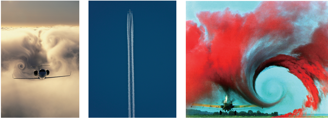
(a) Wake vortices of a Learjet 60 in cloud [2] (b) Wake vortices at high altitude as contrail [3] (c) Wake vortices made visible in a NASA test by using colored smoke rising from the ground [4]
