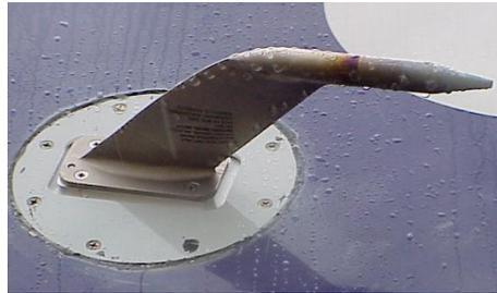
FIGURE 1.5 – Sonde Pitot, design SA/LR.
