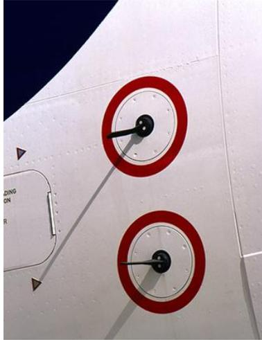
FIGURE 1.7 – Sondes d'incidence, design SA/LR.
