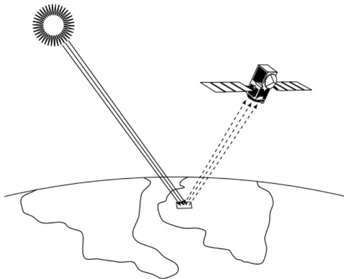
**Figure:** Remote Sensing: The Sun's radiation reflected on the Earth's surface is captured by an airborne or spaceborne hyperspectral sensor.
