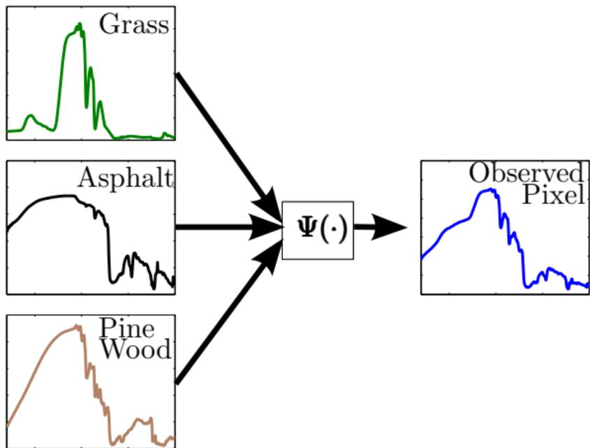
Figure: A observed pixel is in fact a mixture of spectral signatures.
