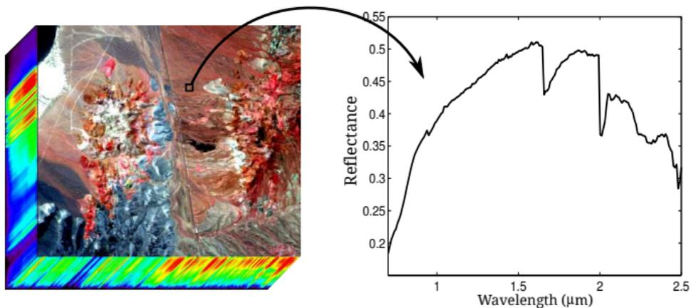
Figure: Illustration of the Hypercube captured by the AVIRIS instrument from the Cuprite field.
