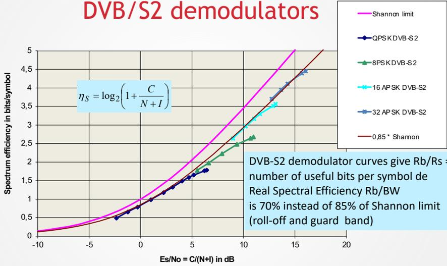
DVB-S2 demodulator curves give  $R_b/R_s =$  number of useful bits per symbol de Real Spectral Efficiency  $R_b/BW$  is 70% instead of 85% of Shannon limit (roll-off and guard band)
