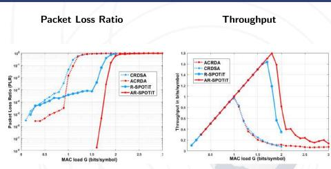
Equipowered packets of 150 symbols, 100 virtual time slots per virtual frame, 3GPP turbo coding of rate 1/3, QPSK modulation, gold code preambles, AWGN channel,  $E_S/N_0 = 10$ dB, 2 replicas/packet.
