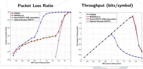
Equipowered packets of 150 symbols, 100 time slots per frame, 3GPP turbo coding of rate 1/3, QPSK modulation Gold code preambles of 31 symbols, AWGN channel,  $E_S/N_0 = 10$ dB, 2 replicas/packet.
