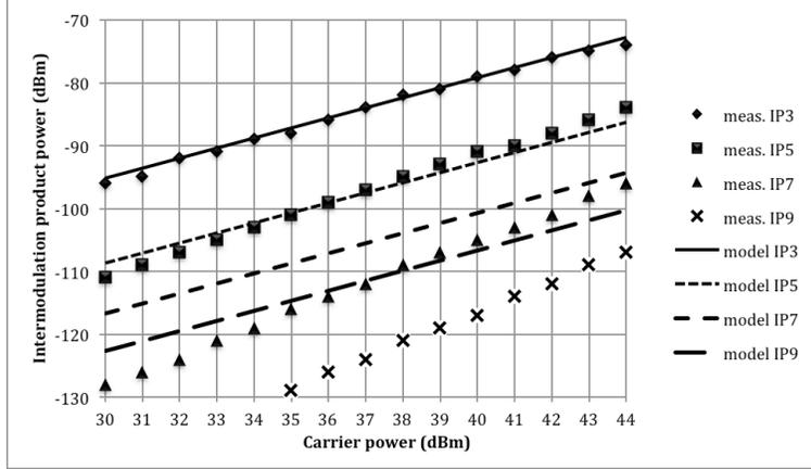
**Figure 1: Comparison of measurement data in [4] with results of a model with one term of degree 1.6**
