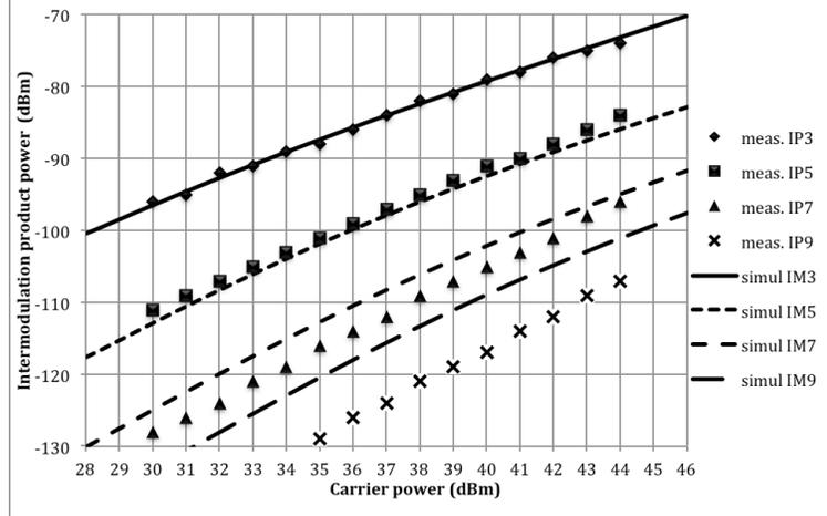
**Figure 3: Comparison of measurement data in [4] with results of a non-analytical Padé-type model**
