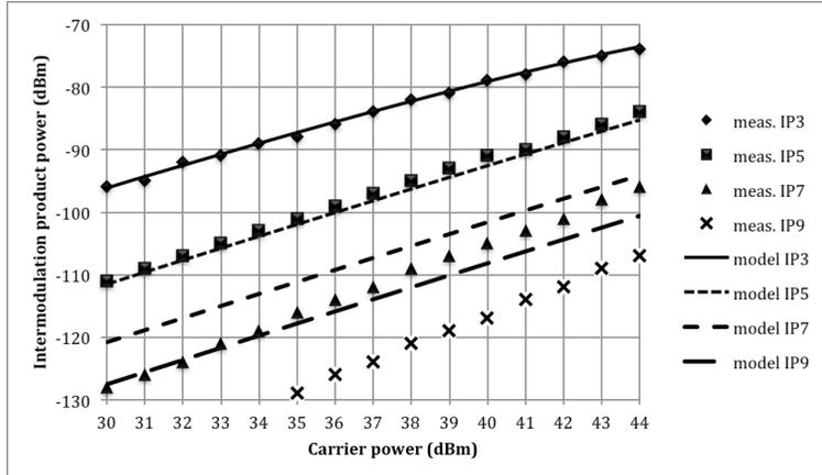
**Figure 2: Comparison of measurement data in [4] with results of a model with two terms of degrees 2 and 2.5**
