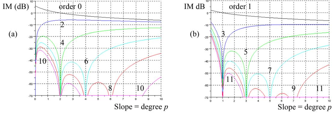
**Figure 4: Multiplicative coefficients versus degree (or IM slope) for the first even orders (a) and the first odd orders (b)**
