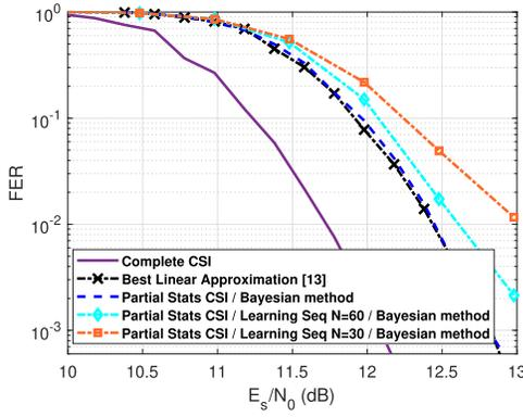
Fig. 4. GPS L1C frame error rate under a Rayleigh channel with  $a = 0.2$ .
