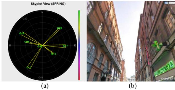
Fig. 6. 6(a) Sky-plot of GPS satellites in the deep urban section (a mask elevation of  $10^\circ$  is applied); 6(b) a street and a sky view of the considered trajectory.
