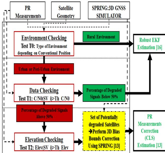
Fig. 7. Positioning Algorithm depending on the environment (“Maps of PR bias Correction Availability”)
