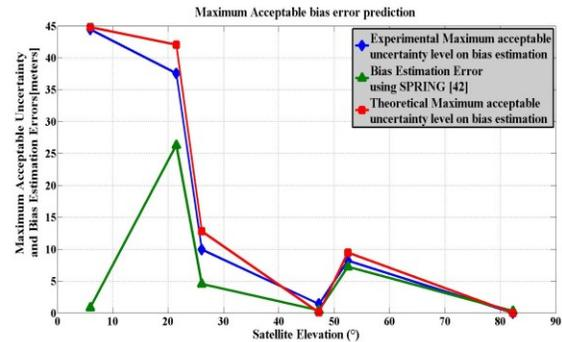
Fig. 5. Experimental maximum acceptable bias estimation uncertainty and bias estimation error using SPRING [23].
