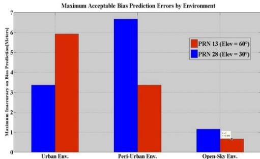
Fig. 4. Experimental maximum acceptable bias estimation uncertainty in different environments for two GNSS satellites.
