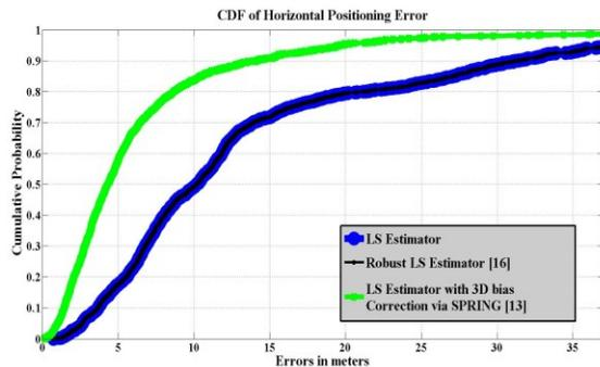
Fig. 8. CDF of horizontal Positioning in deep urban environment using bias correction via 3D GNSS Simulator.
