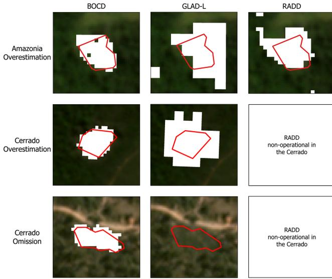
**Fig. 4.** Example of BOCD, GLAD-L and RADD’s detection of MapBiomass Alerta polygons.
