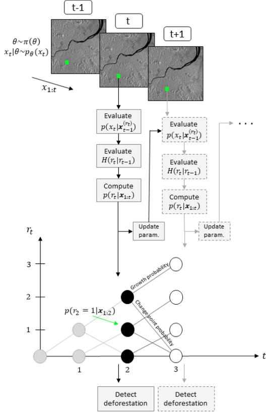
**Fig. 2.** BOCD working principle:  $r_t$  represents the output triangular matrix. The circles indicate probability values for each possible run length, while the colors differentiate past (gray), present (black), and future (white) acquisitions. A significant drop in probability indicates a deforestation event.
