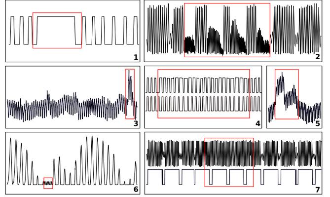
**Fig. 1:** Examples of univariate (1,2,3,5,6) and multivariate (4,7) anomalies in telemetry data (red boxes).
