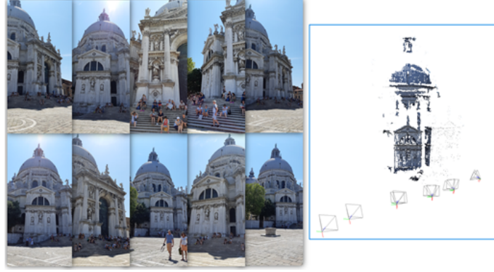
Figure 1.15: Structure from motion example, left: set of images, right: 3D reconstruction using the reconstruction implementation Multi-View Environment [FLG14].
