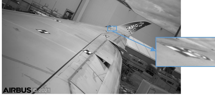
Figure 2.15: Example of view on an A350 wing using a 4K camera, with concentric circular and cross targets installed.
