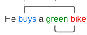
Fig. 3: Example of the attention mechanism for a sentence. A dashed line corresponds to a weak connection between words, whereas a plain line is used for a strong connection.
