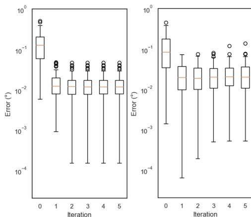
Fig. 5. Angle estimation errors after multiple iterations for the California set with (left) and without (right) uncertainties.
