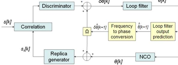
Figure 1: PLL structure with single-frequency phase unwrapping [5]
