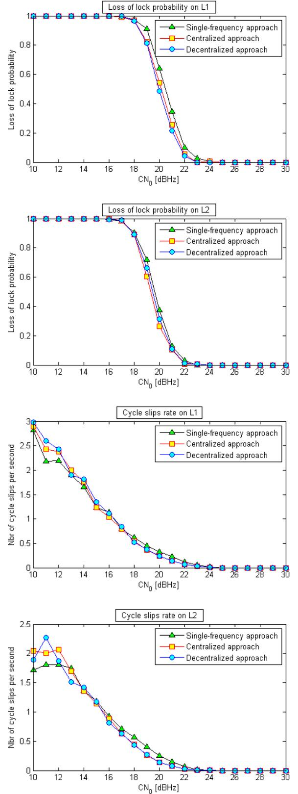
Figure 4: Tracking performance of PLLs with different phase unwrapping structures. Single- vs multi-frequency approaches (L1 and L2 have the same power)
