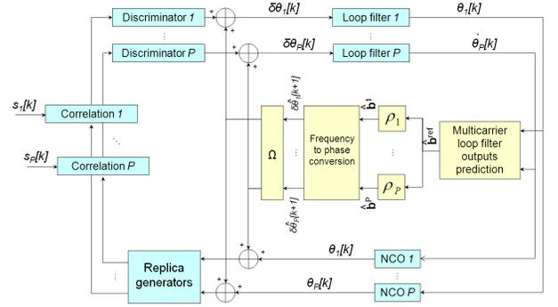
Figure 2: Multifrequency PLL structure in case of a centralized approach
