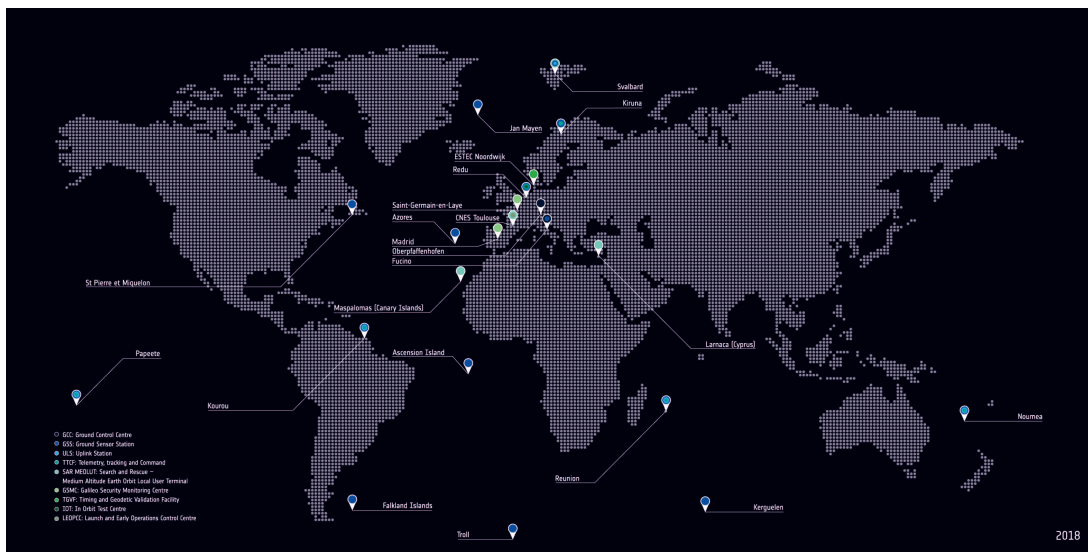
Figure A.3: Galileo Ground Segment: Ground Station Network [16]
