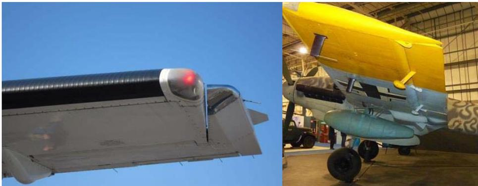
Figure 2.24.: Example of balanced control surfaces (ATR72 and Messerschmitt Bf110).
