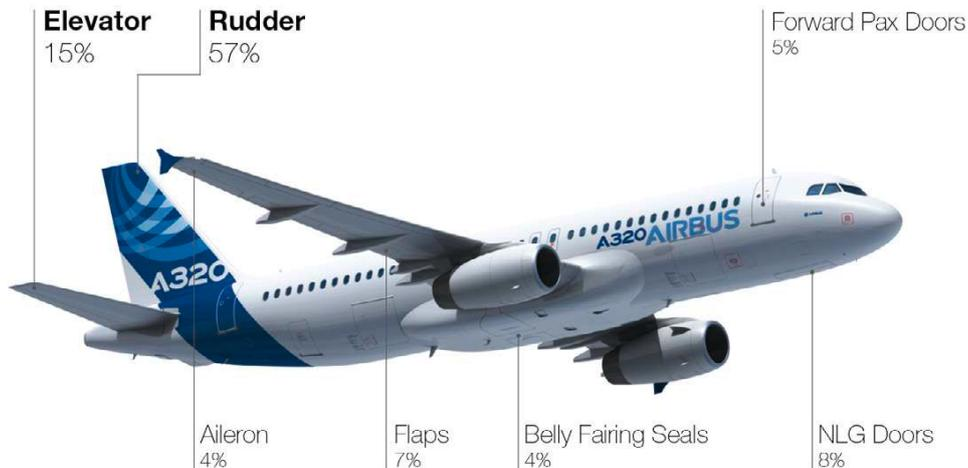
Figure 1.1.: Main sources of vibration on A320 Family aircraft [SAS17].
