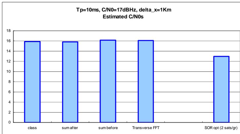
Fig VI-20: Estimated  $C / N_0$  for a signal of 17 dBHz , with fixed  $T_p$
