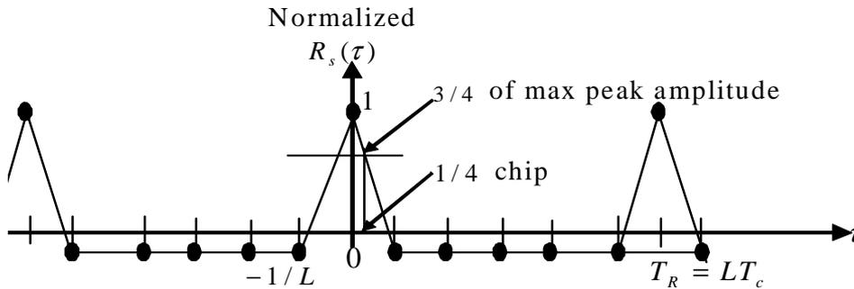
Fig II-8: Degradation of the C/A code autocorrelation function (normalized) for a code phase uncertainty of 1/4 chip
