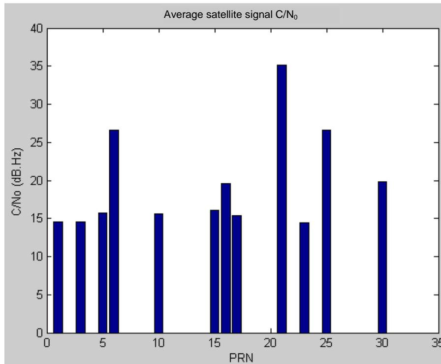
Fig IV-33 : Alcatel demonstrator average satellite signal  $C/N_0$
