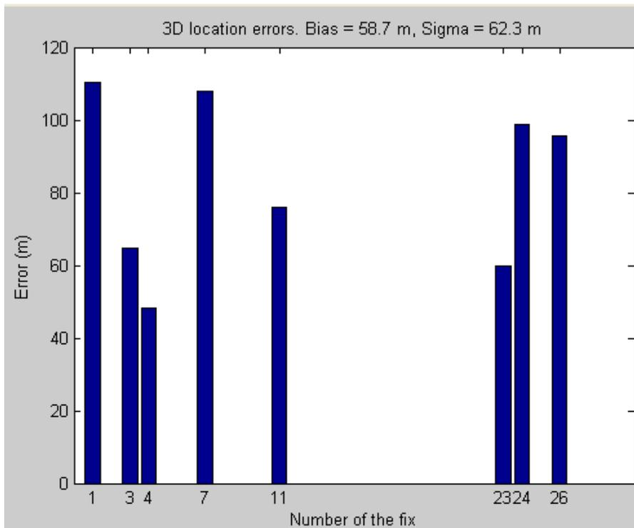
**Fig IV-22 : Alcatel demonstrator 3D position error**
