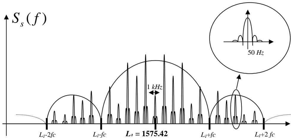
Fig II-3 : PSD of the GPS  $L_1$  transmitted signal
