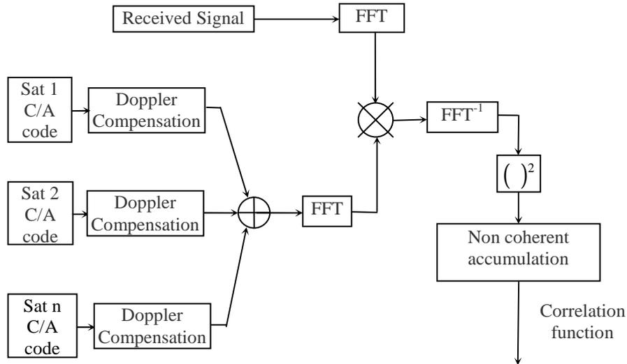
**Fig V-14 : SOR algorithm principle**
