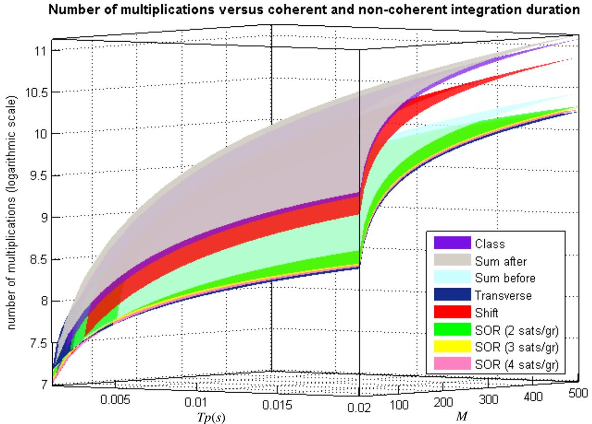
**Fig VI-2 : Number of multiplications carried out during acquisition for the different algorithms, with 9 satellites in view**
