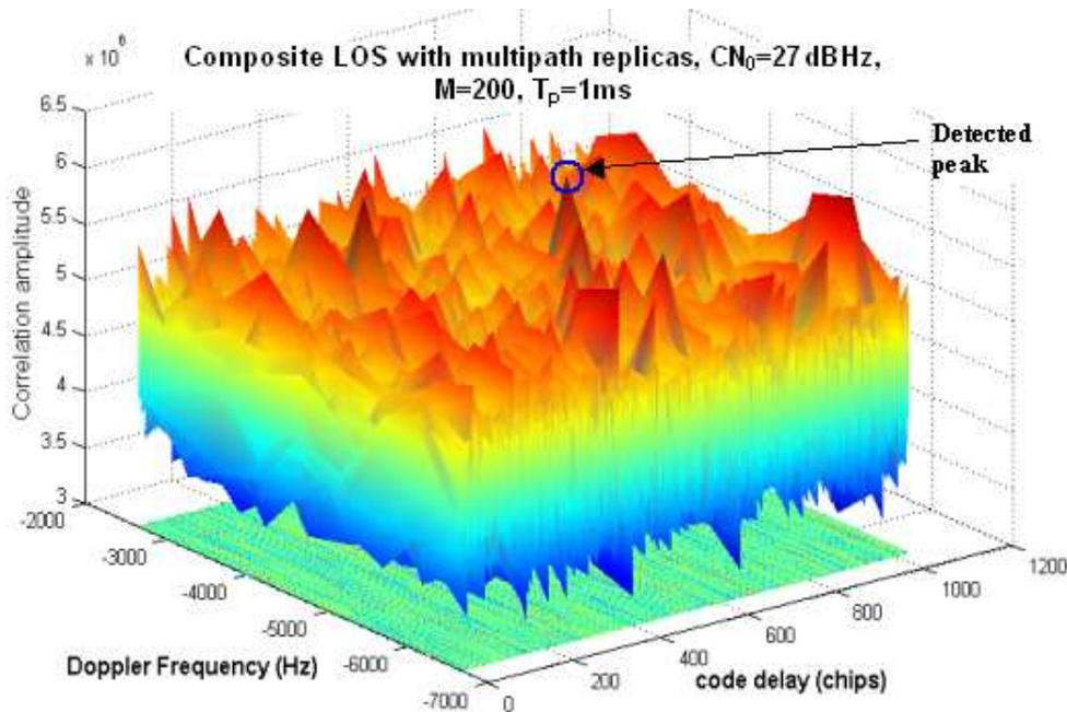
**Fig III-8: Composite LOS with multipath replicas;  $C/N_0 = 27 \text{ dBHz}$  true values: Doppler frequency  $-4666 \text{ Hz}$ , code delay  $608.27 \text{ chips}$ ; estimated values: Doppler frequency  $-4666 \text{ Hz}$ , code delay  $608.27 \text{ chips}$ ,**
