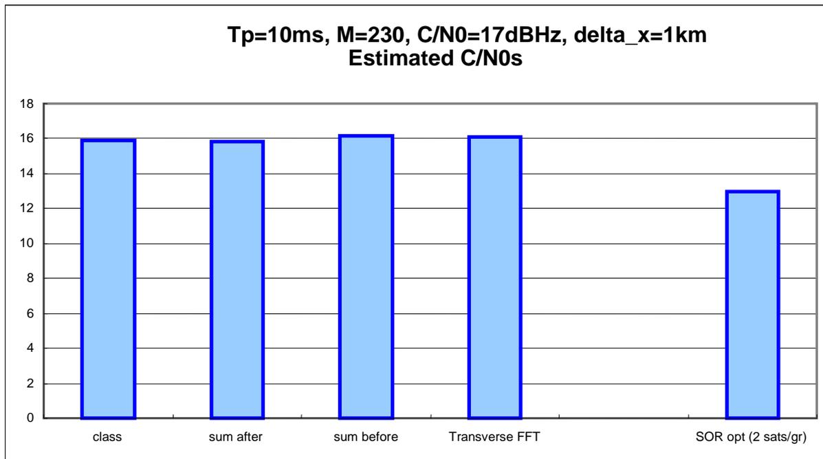
Fig VI-13: Estimated  $C/N_0$  for a signal of 17 dBHz, with fixed  $M$  and  $T_p$
