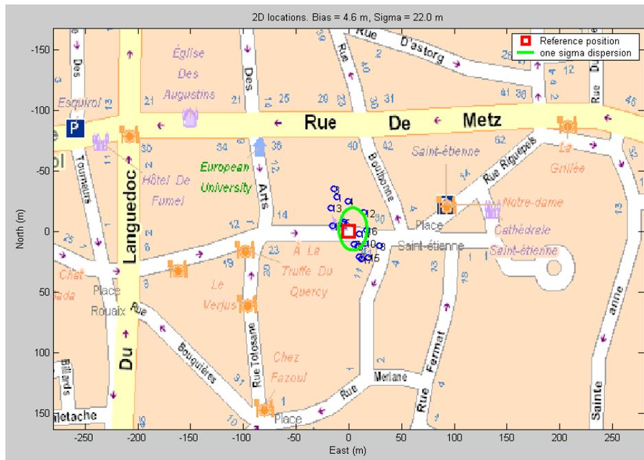
Fig IV-26 : Alcatel demonstrator 2D error
