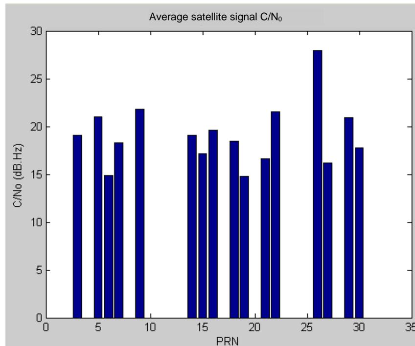
Fig IV-23 : Alcatel demonstrator average satellite signal  $C/N_0$
