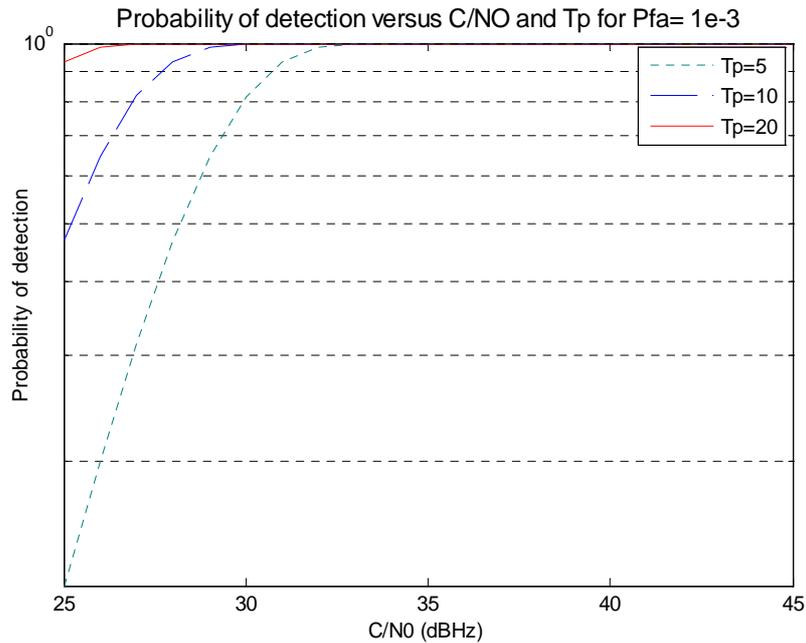
**Fig II-12: Probability of detection for a Probability of false alarm equal to  $10^{-3}$ ,  $M = 5$  and  $T_p = 5\text{ ms}$ ,  $T_p = 10\text{ ms}$  and  $T_p = 20\text{ ms}$  respectively**
