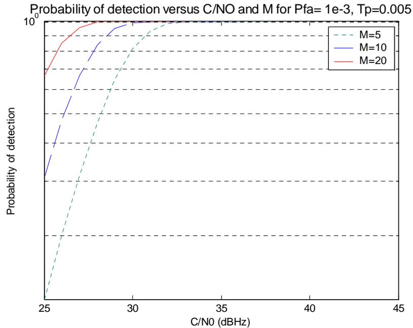
**Fig II-11: Probability of detection for a Probability of false alarm equal to  $10^{-3}$ ,  $T_p = 5\text{ms}$  and  $M = 20$ ,  $M = 10$  and  $M = 5$  respectively**
