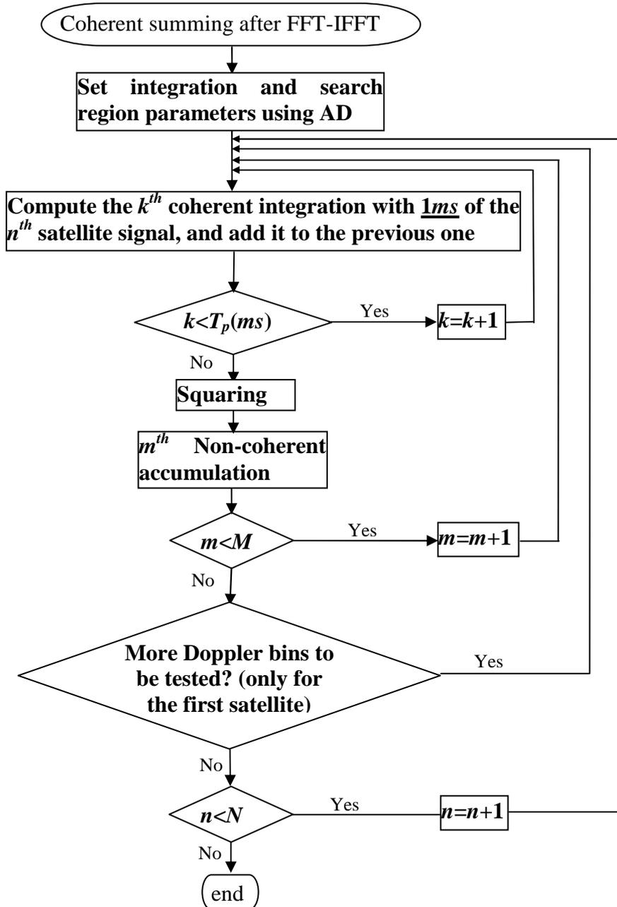
Fig V-7 : Coherent summing after FFT-IFFT algorithm flowchart
