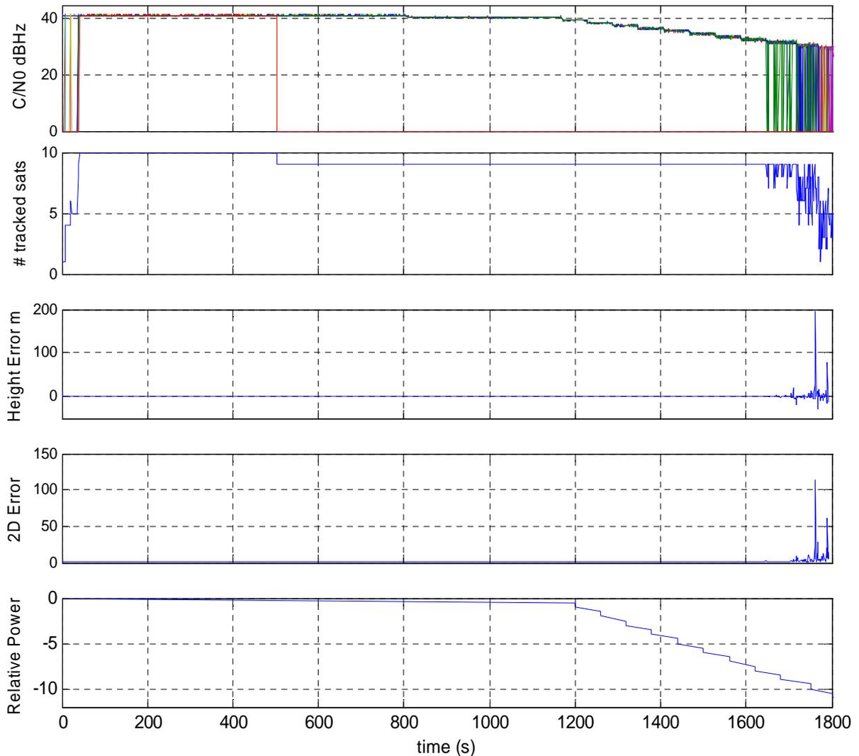
**Fig IV-34 : Tracking performance of a standalone receiver (OEM4)**
