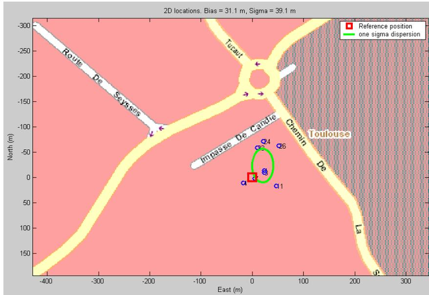
**Fig IV-21 : Alcatel demonstrator 2D position error**
