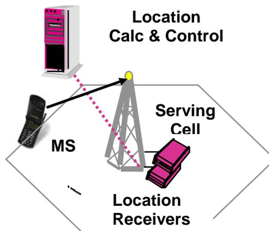
**Fig. D-6: Multipath fingerprint wireless location technique [Rossati, 2001]**
