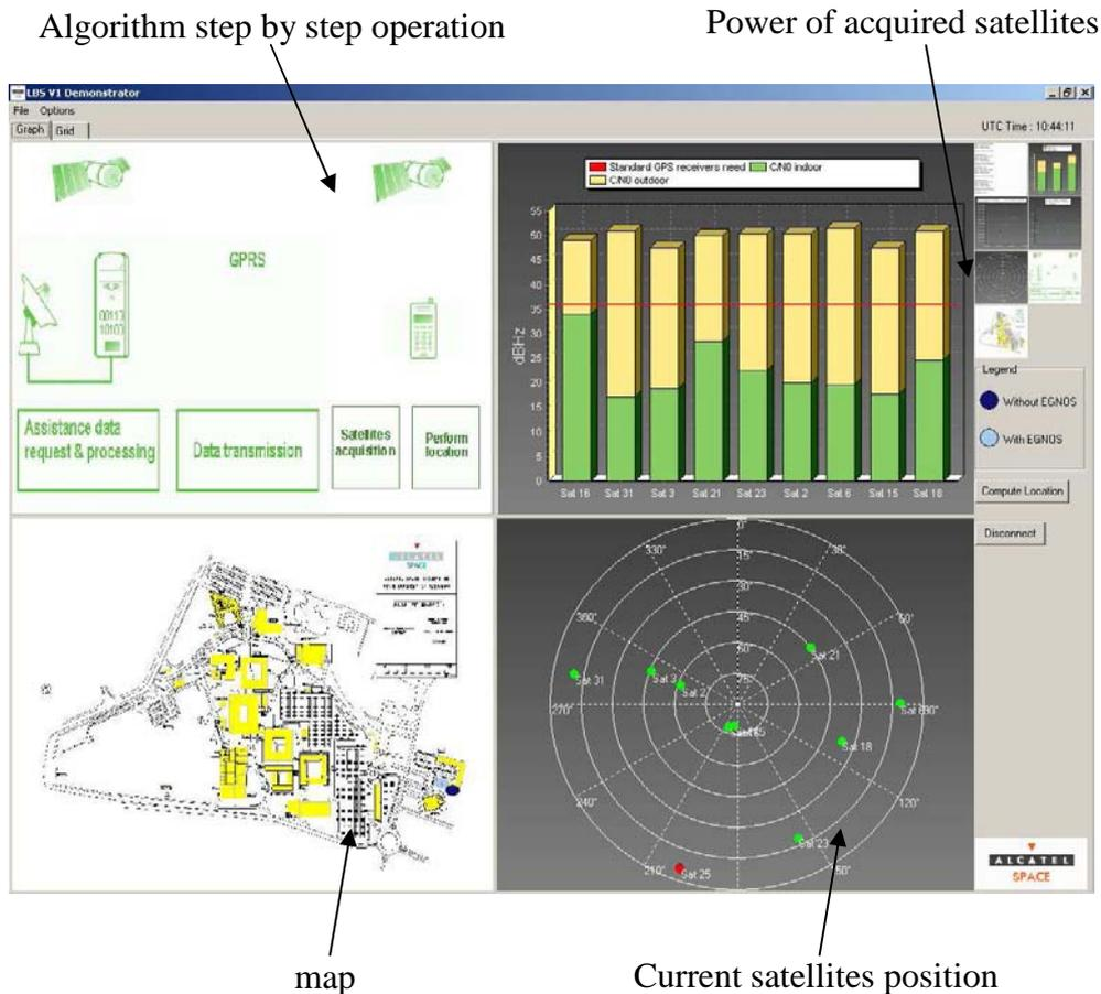
Fig IV-10 : Graphical interface of the Alcatel AGPS receiver
