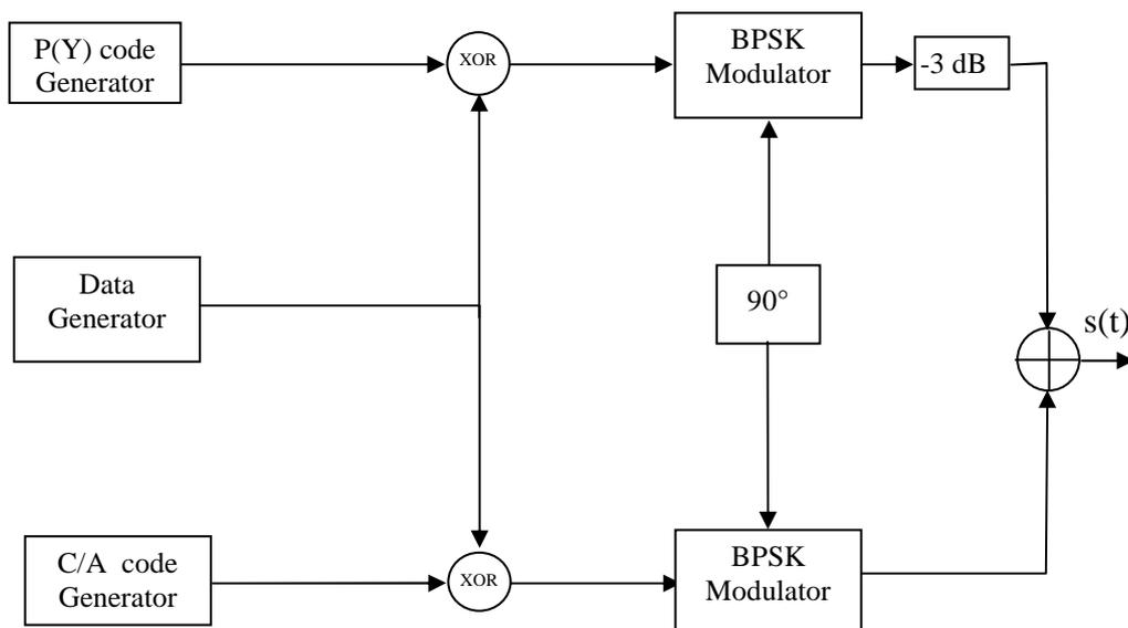
**Fig II-2: GPS  $L_1$  carrier modulation**
