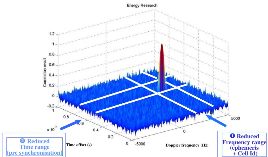
**Fig IV-6 : Reduction in the search space using the AGPS Assistance Data**
