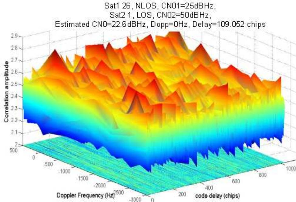
**Fig III-12: Cross-correlation between 2 GPS signals: 1- Non LOS signal of satellite number 26 (just multipath replicas), true Doppler 4000 Hz , true delay 604.03 chips, initial  $C/N_0 = 25$  dBHz 2- LOS signal of satellite number 1 with multipath replicas, true Doppler 0 Hz , true delay 608.27 chips, initial  $C/N_0 = 50$  dBHz .**
