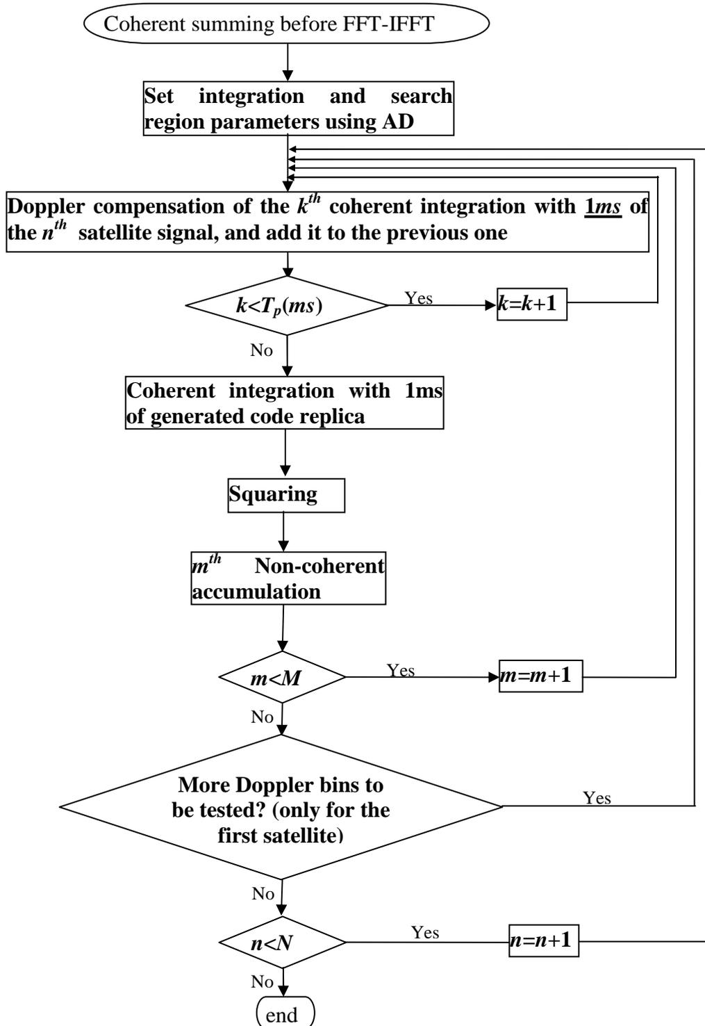
Fig V-8 : Coherent integration by summing before FFT-IFFT algorithm flowchart
