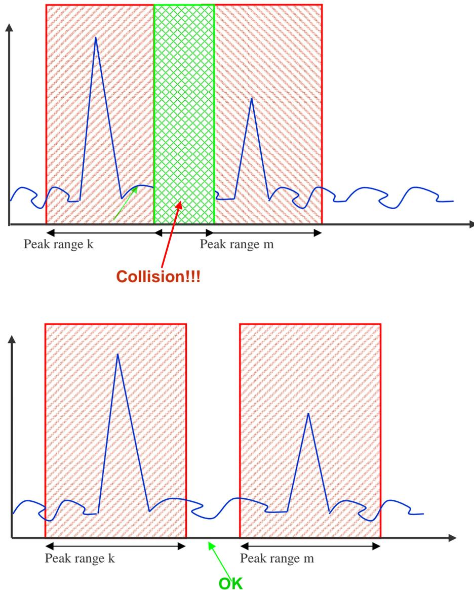
**Fig V-17 : Collisions between satellites having close code delays**
