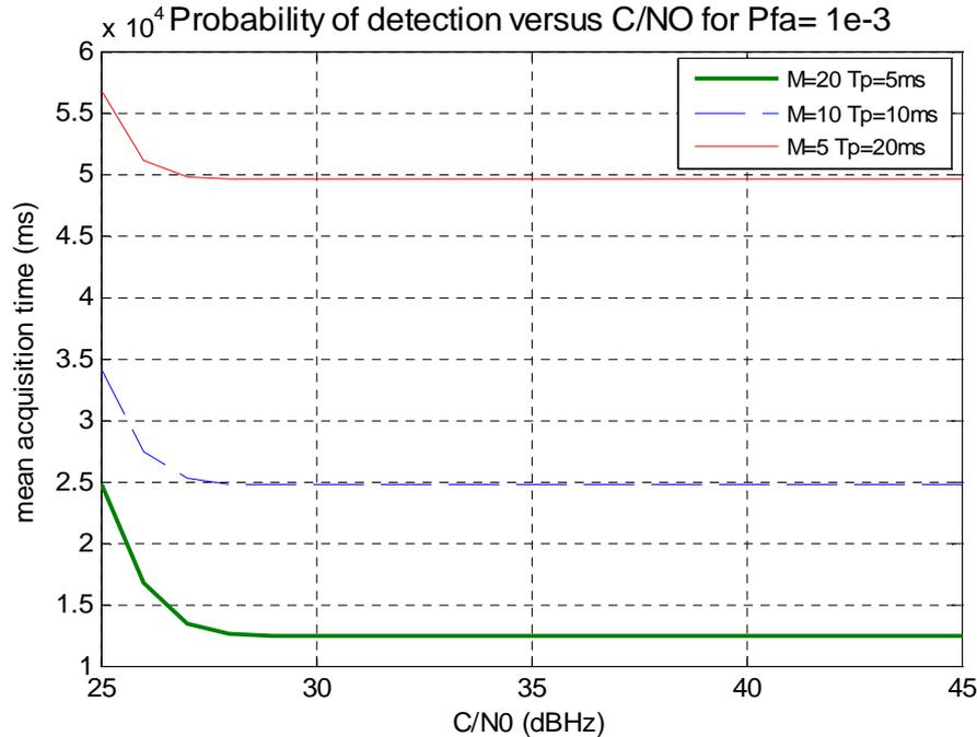
**Fig II-18:** Mean acquisition time (in ms) versus  $C/N_0$  (dBHz) for a constant dwell time and  $p_{fa} = 10^{-3}$
