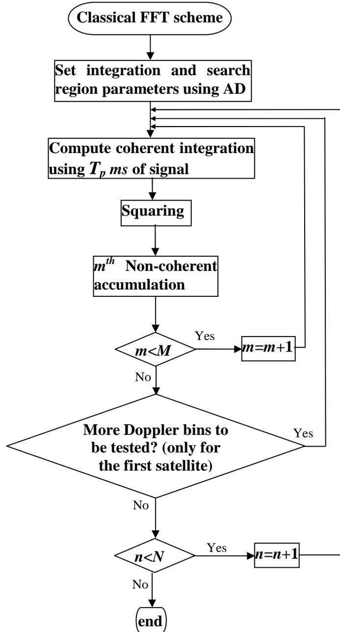
Fig V-3 : Classical acquisition algorithm flowchart
