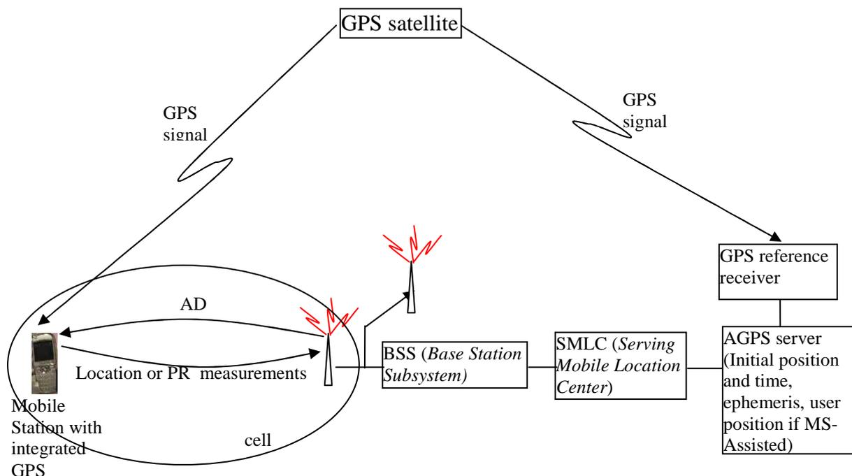
Fig IV-5 : General AGPS functioning process
