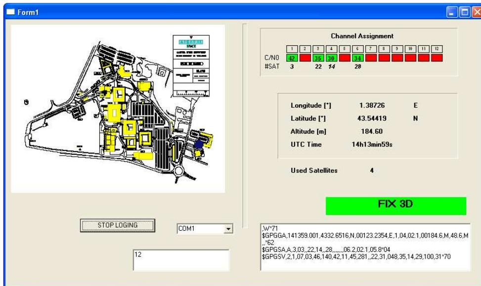
Fig IV-9 : Graphical interface of the Haicom receiver
