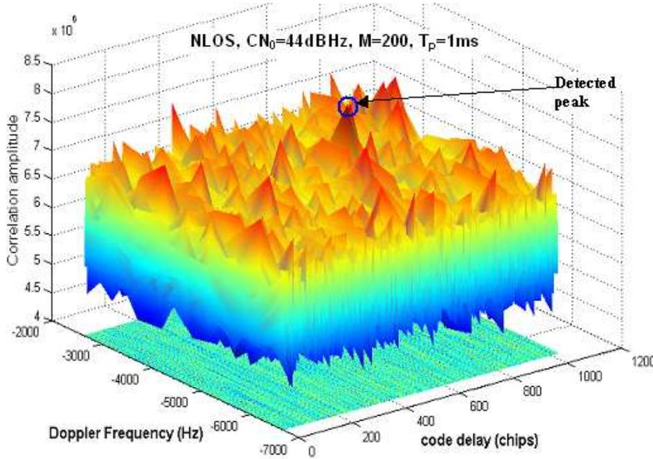
**Fig III-9: NLOS signal, multipath replicas only;  $C/N_0 = 50 \text{ dBHz}$  ( $C/N_0$  of the LOS that could not reach the receiver); true values (of the LOS): Doppler frequency  $-4666 \text{ Hz}$ , code delay  $608.27 \text{ chips}$ ; estimated values: Doppler frequency  $-4666 \text{ Hz}$ , code delay  $608.27 \text{ chips}$**
