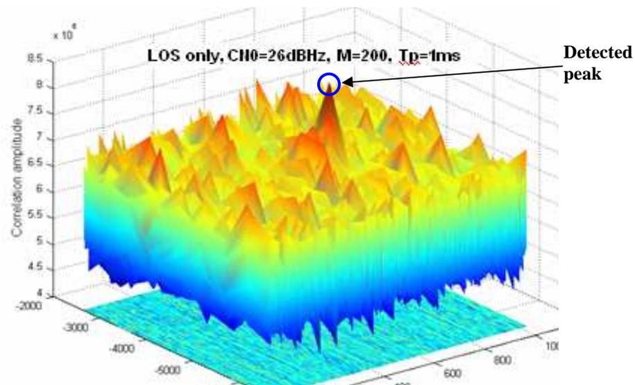
**Fig III-7: LOS without multipath replicas;  $C/N_0 = 26\text{ dBHz}$ ; true values: Doppler frequency  $-4666\text{ Hz}$ , code delay  $608.27$  chips; estimated values: Doppler frequency  $-4666\text{ Hz}$ , code delay  $608.27$  chips**
