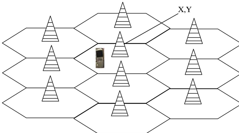
Fig. D-1 : Cell ID wireless location technique
