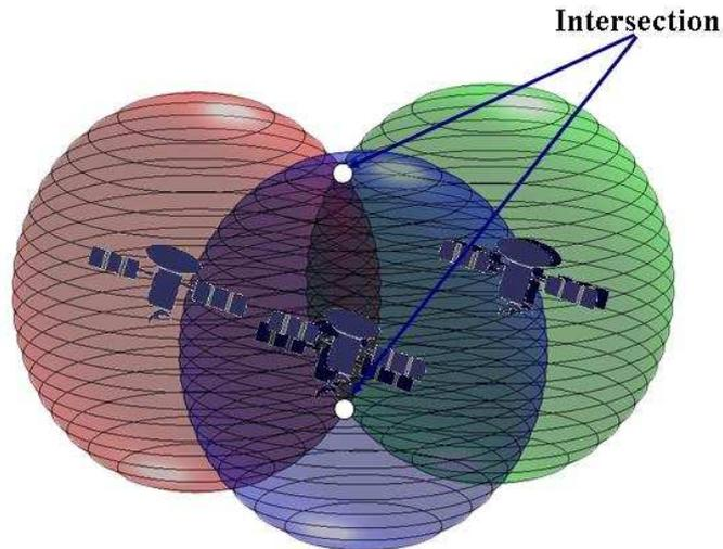
**Fig II-1: The triangulation method for determining the user position**
