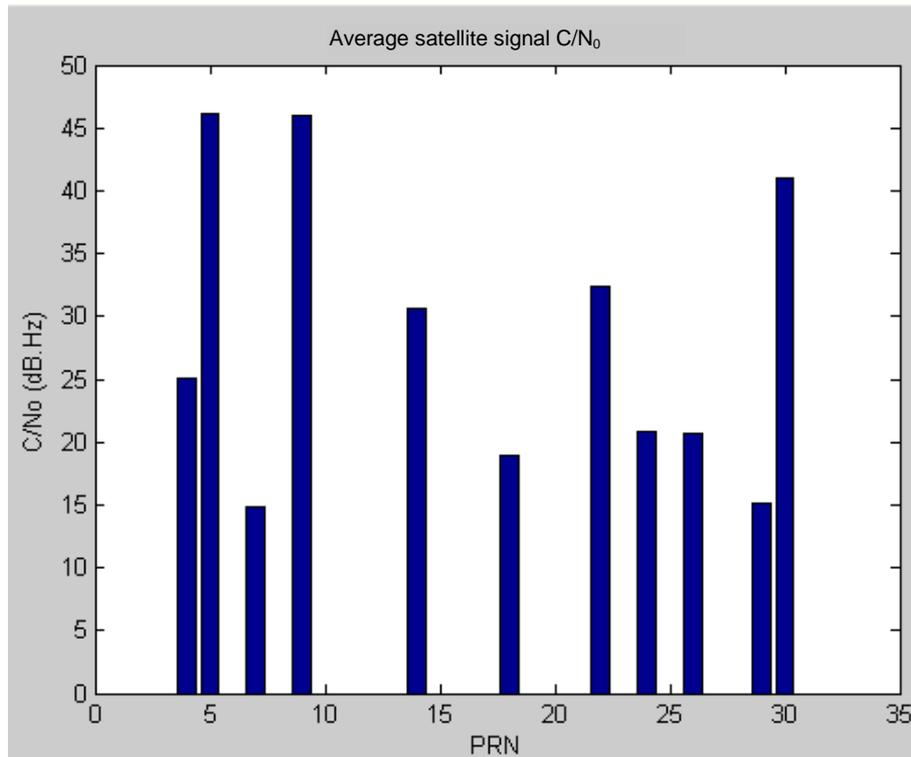
Fig IV-28 : Alcatel demonstrator average satellite signal  $C/N_0$
