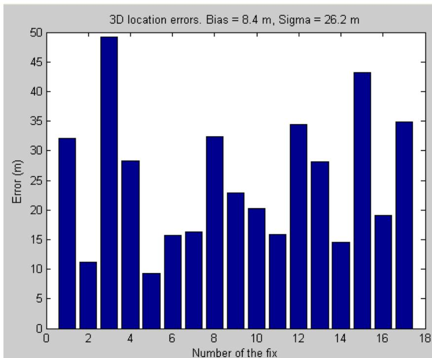
Fig IV-27 : Alcatel demonstrator 3D error
