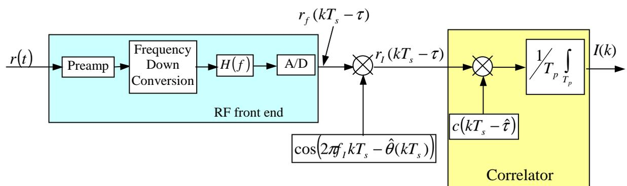
Fig II-4 : GPS received signal demodulation block diagram
