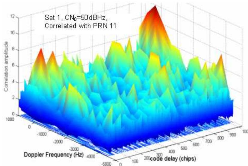
**Fig III-11: LOS signal of satellite number 1 without multipath replicas or noise, true Doppler 0 Hz , true code delay 608.27 chips, signal correlated with C/A code of satellite number 11. Estimated values: Doppler frequency 0 Hz , code delay 980.03 chips**
