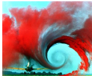
Wake vortices made visible in a NASA test by using colored smoke rising from the ground
